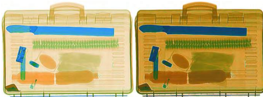
Fig 5.7 Enhancing Effect of Color Image/Low Penetrating Power
