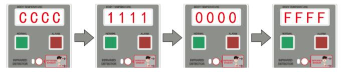
2. Press the adjustment key to enter the volume setting interface. Press the adjustment key to adjust the number. Press the selection key to switch to the reserved function item, the temperature unit selection item and the low temperature voice alarm switch item in turn. You can adjust the value by pressing the adjustment key. After the setting is completed, press the confirmation key to return to the main interface.
