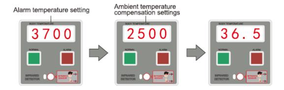
Note: 1) "3700" means the alarm temperature is 37°C.
