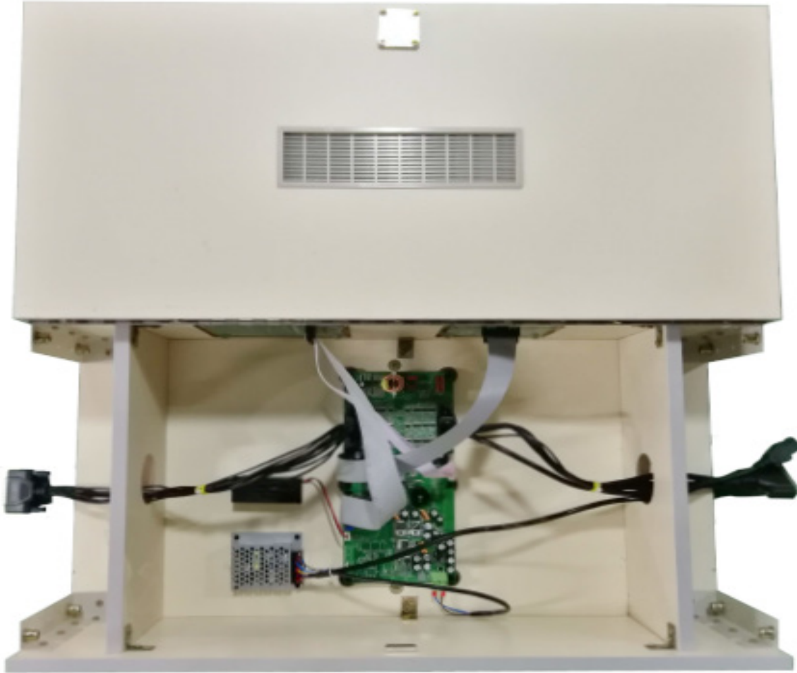
Mother Board + Switch power supply + Zone LED PCB + Keyboard PCB + Speaker
