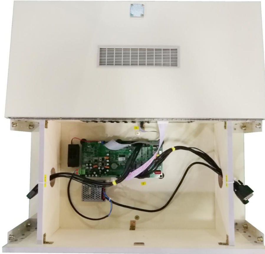
Motherboard +Switch power supply+ LCD + Lamp panel+ Speaker
