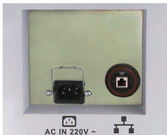
Fig 4.1 Power Supply Connection Position
