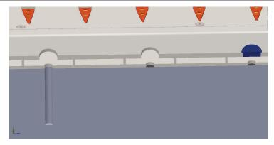
After all holes are finished as required above, the holes are nailed into the prepared chemical bolts (chemical bolt construction process) or expansion bolts.
